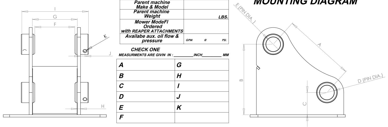
Due to the large range of machine, makes, models and designs on the market this Mount diagram must be completed by the customer to insure that Reaper Attachments proivides you with an accurate mount that fits your Specific type of machine. It is our customers responsability to ensure that all dimensons, provided are correct. Future modifications to mounts that are different than Originally specified by the customer will be at an added expense.
